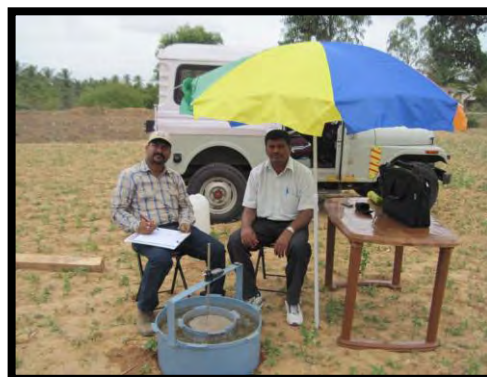
Fig-2.1 Soil Infiltration test in progress in Micro level area of Tumkur district(Karnataka)
