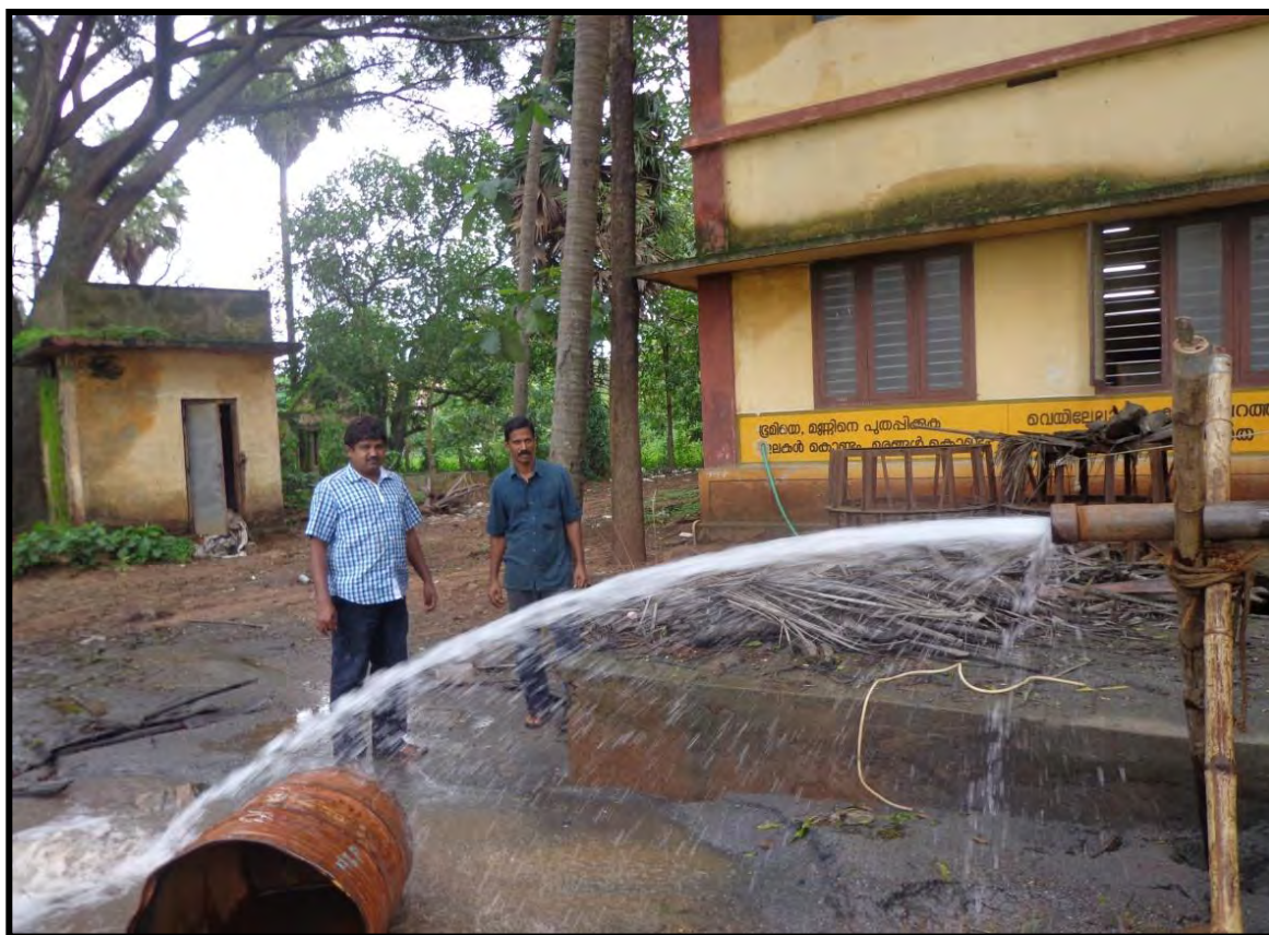
Fig 4.2 Aquifer Performance Test of EW at Vadakarapathy Panchayat Office, Nallur, Palakkad district.
