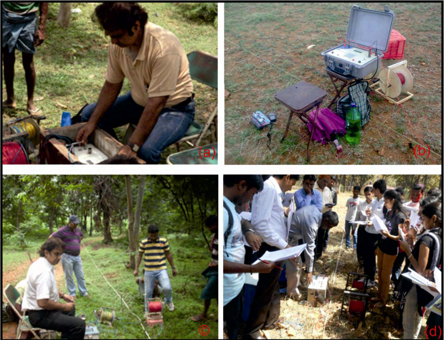
Fig-5.1 (a) Resistivity survey with the CRM – 500 instrument in the SFTI campus, Gaya (b) Resistivity survey in Aquifer mapping area, Kolar District (c) Arrangement for VES with Syscal R2 resistivity meter in deer (Mrig) park, Rajgir. (d) Demonstration of Geophysical survey to the trainees during Training Programme (March 2014)
